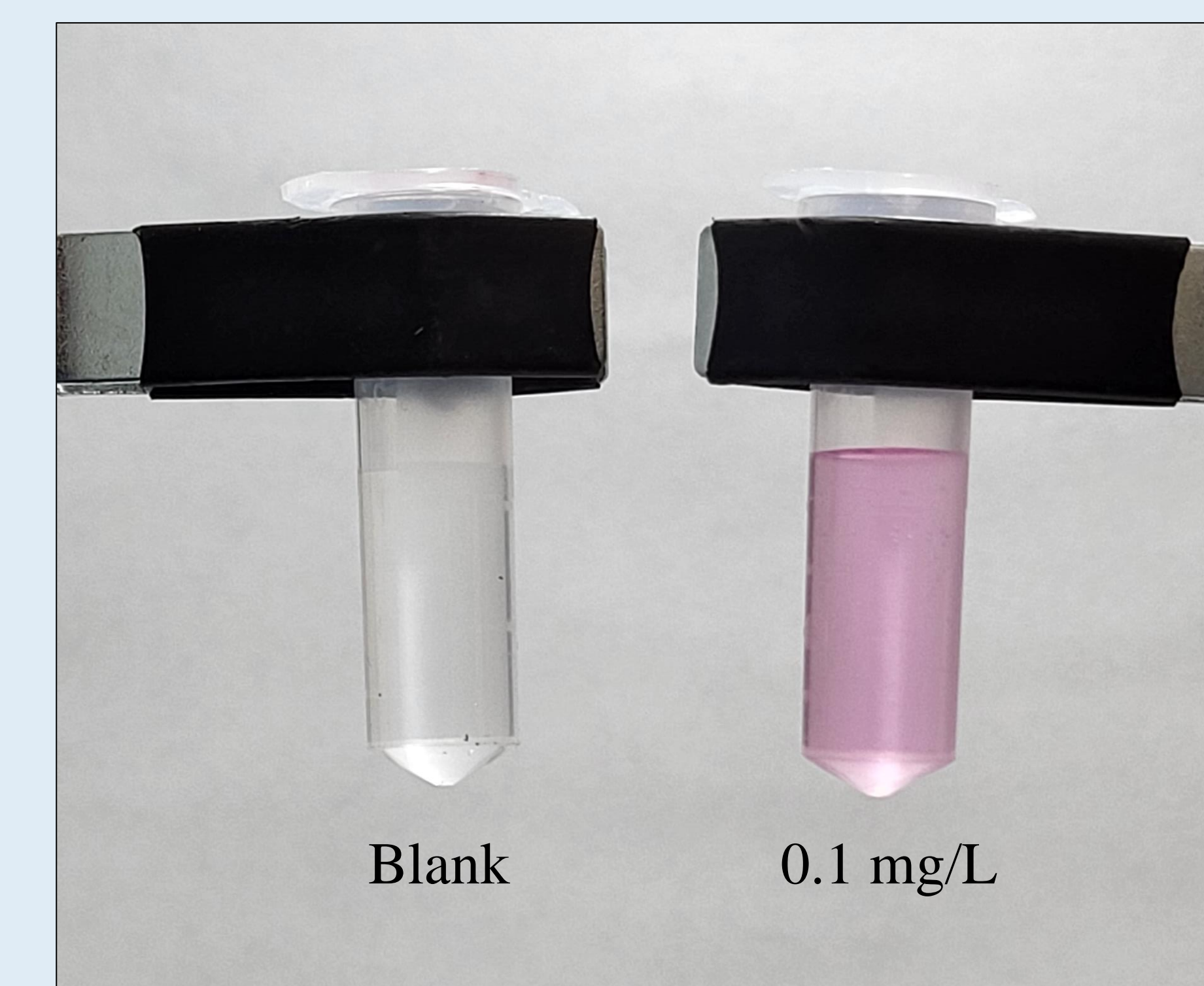
Fig. 4. Preliminary results of the tablet sensor for nitrite detection in water.
